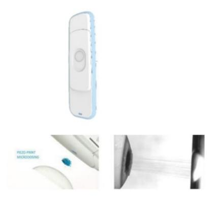
The Optejet dispenser delivers doses of  $6-8 \ \mu$ L, directly coating the corneal surface where 80% of intraocular drug penetration occurs. We believe that microdosing may reduce drug and toxic preservative exposure by more than 75%, thus reducing ocular irritation, and resulting in potentially gentler treatments without compromising the desired clinical effect. Our approach could also reduce inadvertent waste associated with poor administration of conventional macrodose drops.
