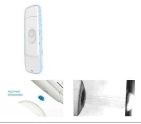
The Optejet dispenser delivers doses of  $6-8 \mu$ L, directly coating the corneal surface where 80% of intraocular drug penetration occurs. We believe that microdosing may reduce drug and toxic preservative exposure by more than 75%, thus reducing ocular irritation, and resulting in potentially gentler treatments without compromising the desired clinical effect. Our approach could also reduce inadvertent waste associated with poor administration of conventional macrodose drops.
